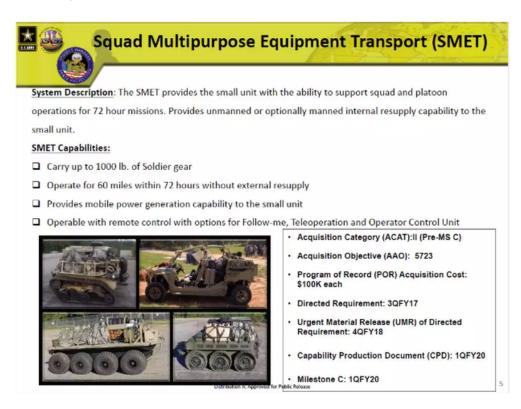
Besides hauling soldiers' heavy gear packs, MUTT can hold anti-tank missiles and or spare ammunition.
