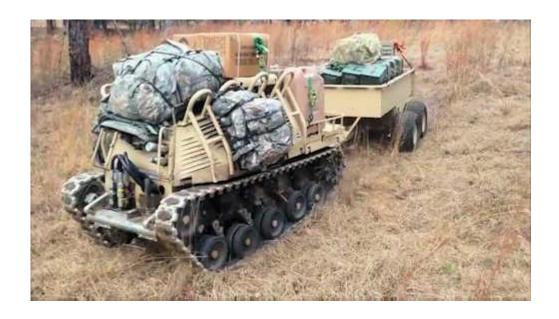
MUTT comes in several sizes: tracked,  $6\times6$ , and  $8\times8$ . It measures 9 feet long by 5 feet wide, can carry 1,000 pounds of gear, and also provide 3,000 watts of power, in addition to a 60-mile range.
