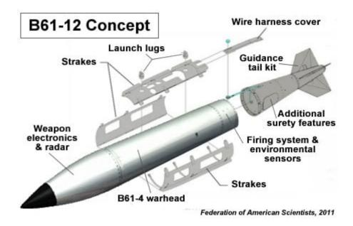
This weapon is built for transport by high-speed fighter aircraft. The casings are streamlined in order to be compatible with supersonic travel. The weapons are 11 feet by 8 inches (3.56 m) long. The diameter is approximately 13 inches (33 cm). This ordnance typically weighs 700 pounds (320 kg) although they could have different sizes depending upon the
