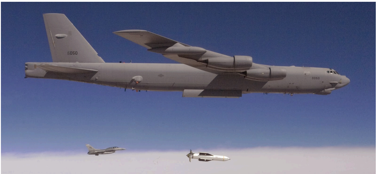
B-52 dropping a MOP escorted by an F-16 during a test trail.
