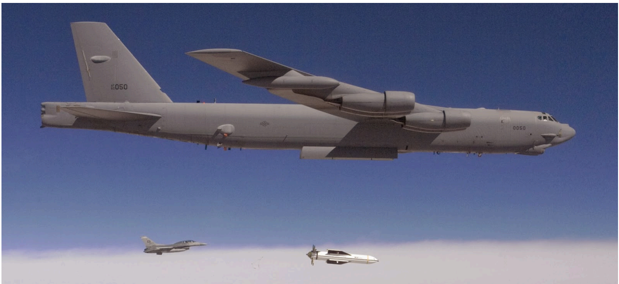
B-52 dropping a MOP escorted by an F-16 during a test trail.
