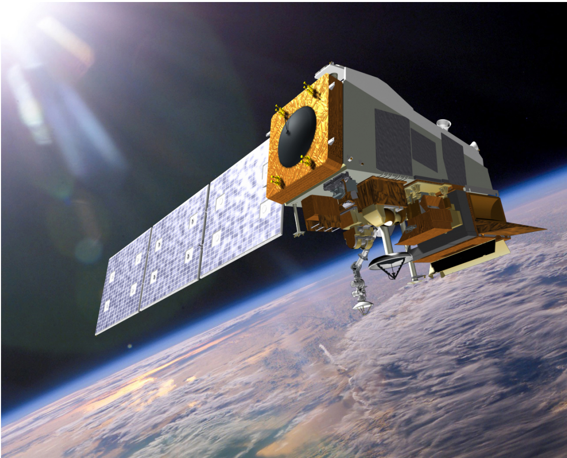
The Suomi National Polar-orbiting Partnership (Suomi NPP) satellite operated NASA and NOAA detects fires on earth through infrared sensing. Artist rendering via NASA.
