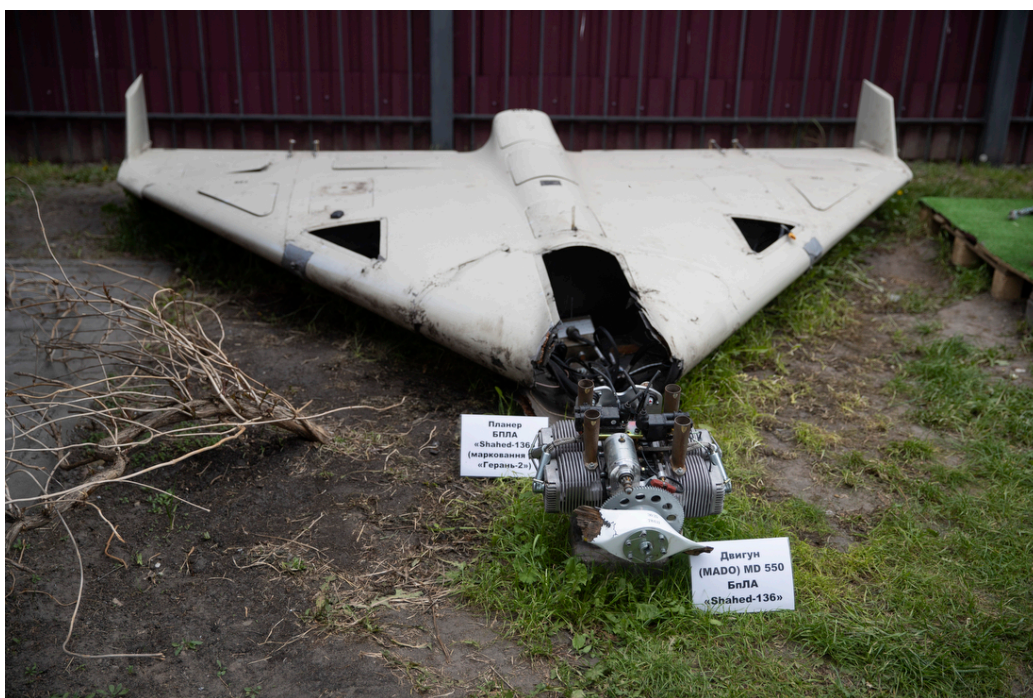
Remains of Shahed 136 and its engine in Kyiv Scientific Research Institute of Forensic Expertise (Licensed under CC BY 4.0)
