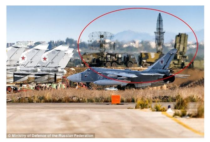
It's operative at a moment's notice, able to simultaneously engage up to 36 targets with up to 72 missiles. Three separate types are used – extremely long range 40N6, long range
