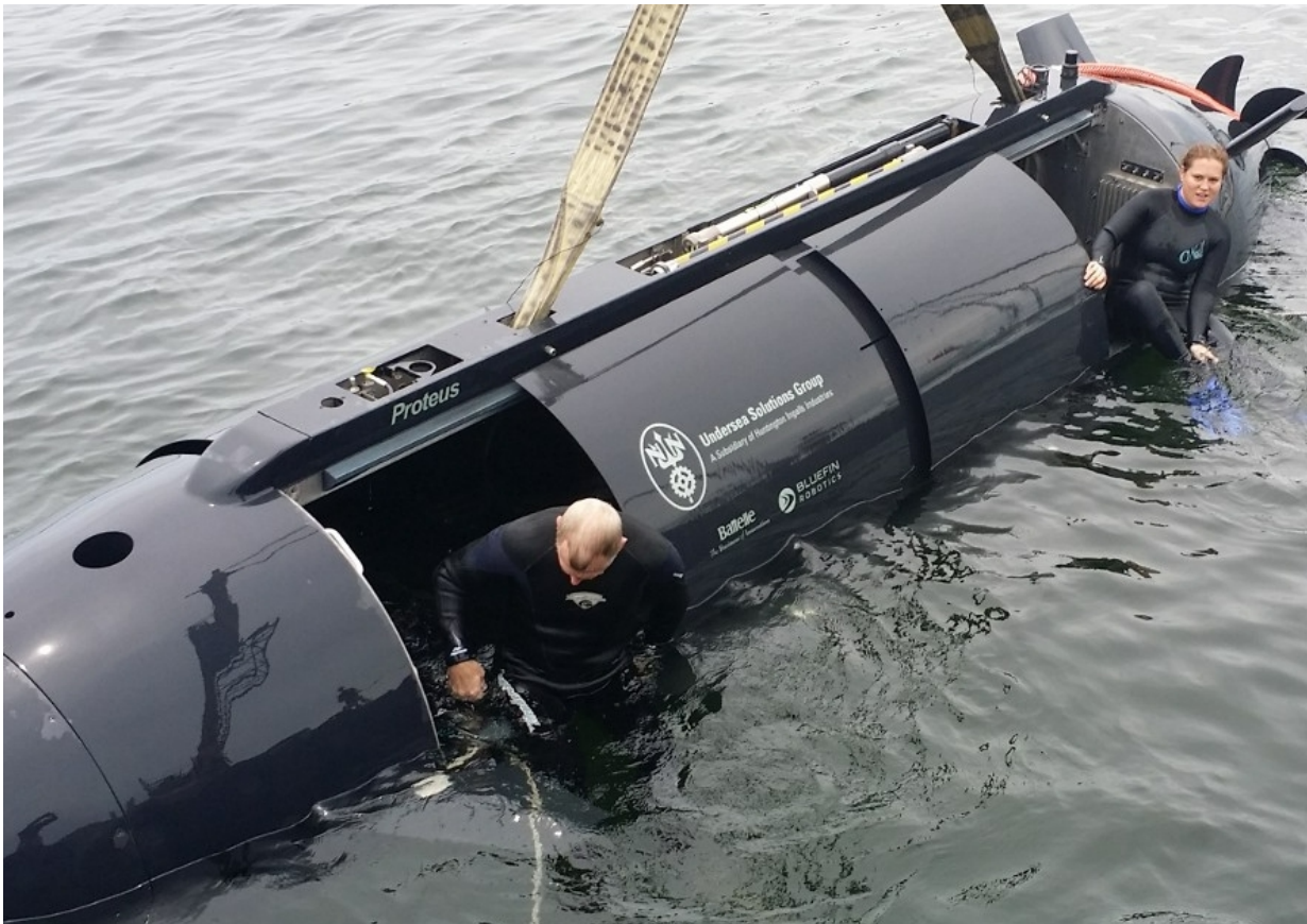
PROTEUS Dual-mode underwater vehicle (DMUV) taken out for a test in Florida's Saint Andrews Bay – USG Vice President Ross Lindman as the pilot is preparing to crew and drive the Proteus dual-mode underwater vehicle. Photo by Joe Colamaria/HII ( source ).
