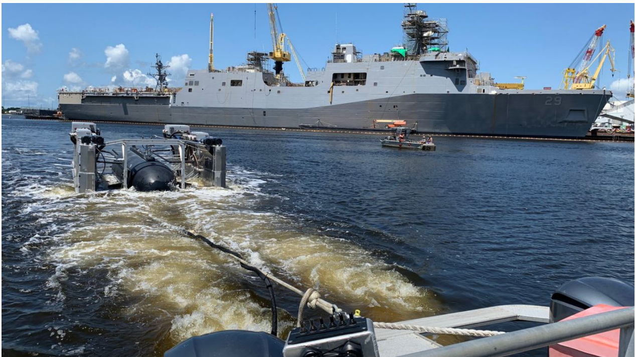
HII's Pharos prototype platform being towed behind a small craft in the Pascagoula River while recovering HII's Proteus LDUUV.
