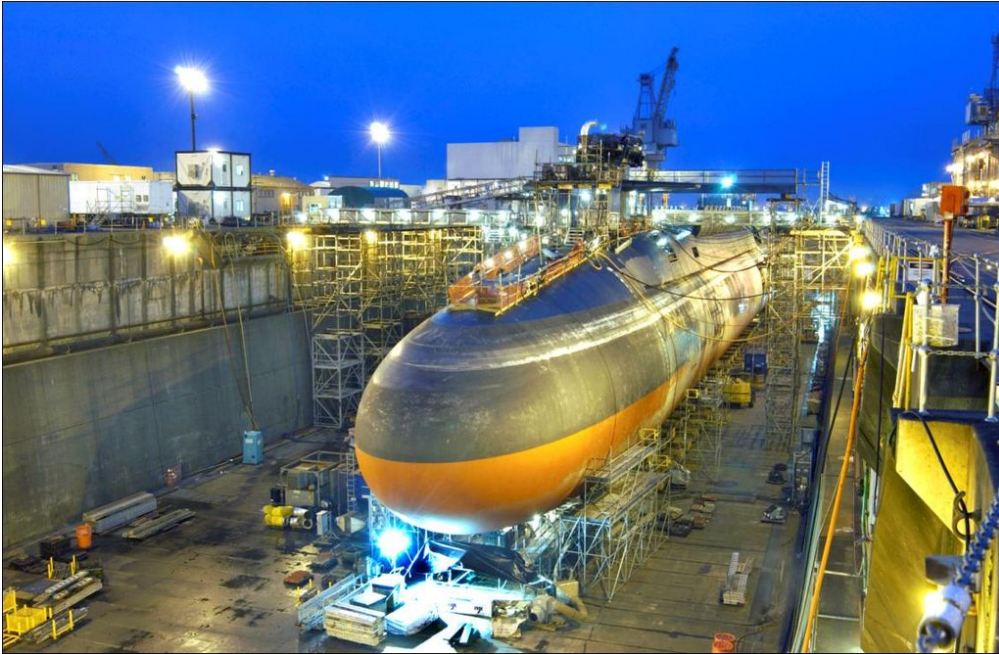
USS Ohio being converted from an SSBN to an SSGN in March 2004 (Source: U.S. Navy photo by Wendy Hallmark)
