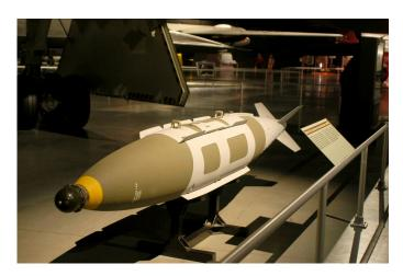
It is also important to note here that the JDAM kit relies on a GPS-assisted inertial navigation system (INS), which means the INS portion of the bomb must ensure that accuracy is retained up to a significant extent, even if the GPS signal is jammed or otherwise lost.
