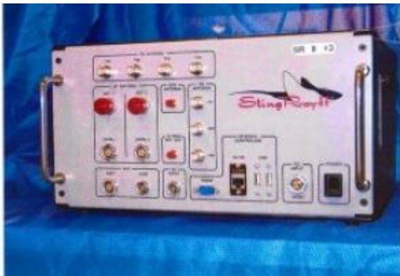
StingRay cell phone spying device (US Patent photo)
