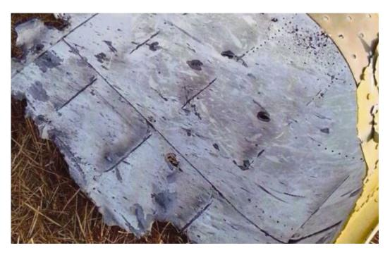
The holes in the wreckage of Malaysia Airlines flight MH17 are believed to have come from 30mm cannon fire.
