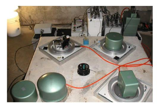
The seismic recording equipment installed in the underground vault. The sensors rest on the central pier, which is directly attached to the coral that underlies the vault so that the instruments can best record the shaking caused as seismic waves travel through the earth.
