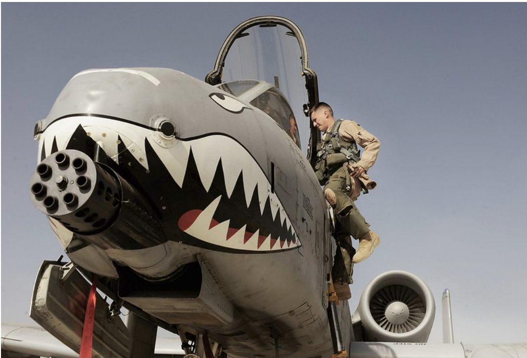
The gatling gun on an A-10 Warthog. (Photo: Willard E. Grande II / USAF)
