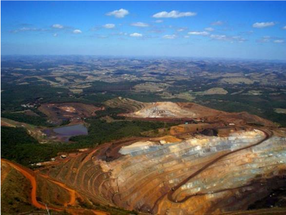
The open pit mine at Brumadinho, Brazil as it appeared in 2008. The waste generated at this mine was stored in nearby tailings lagoons, two of which burst on Jan 25, 2019 after 4 years of dormancy.
