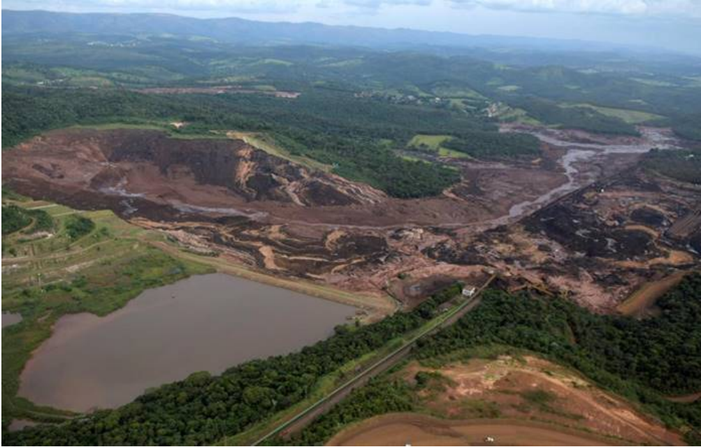
An overview of the massive partially emptied-out tailings lagoon (upper left). Note the slightly smaller, still-intact, water/sludge-filled tailings lagoon (lower left). The downstream devastation is represented in the right side of the photo.
