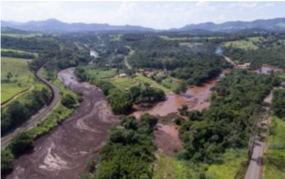
Downstream from the tailings dam. Note the tributary to the right that flows into the main river was heavily contaminated when the flow reversed.
