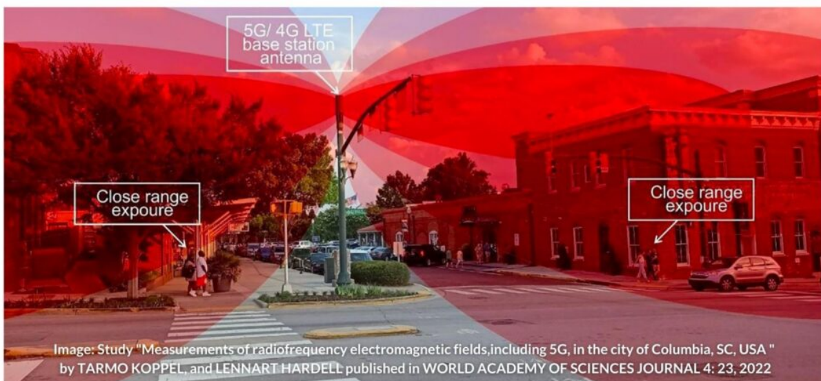
Figure 7. Gervais Street: Cell phone base station antenna placed close to street level and causing high exposure to pedestrians and nearby café visitors (exposure scenario illustration). The antenna appears camouflaged and seemingly part of a utility pole. The measurer only discovered the antenna due to the high radiofrequency levels in the vicinity.
