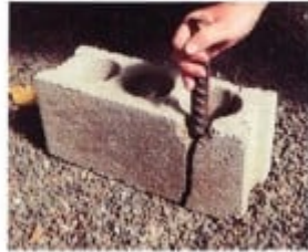
Example of the typical, locally handmade, 400 psi masonry block used for the housing units
