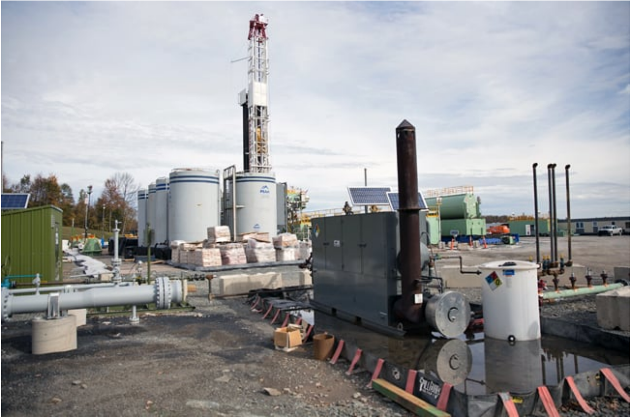
A gas production unit (foreground) cleans, depressurizes, and moderates gas temperatures at a Cabot Oil & Gas drill site in Kingsley, Pa. Photo credit: Lindsay Lazarski/WHYY
