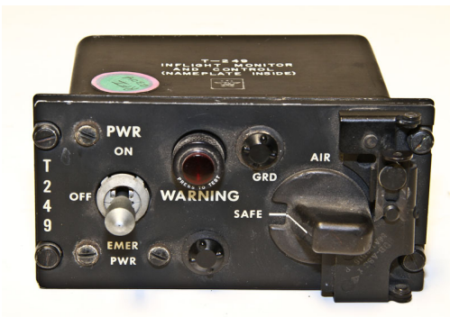
The T-249 switch used to arm nuclear bombs on Strategic Air Command bomber aircraft. Photo courtesy of Glenn's Computer Museum
