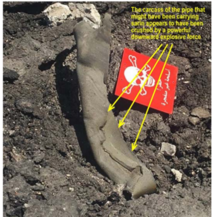
Deformation of sarin containing pipe and crater from the action of the explosive charge placed on top of the sarin containing pipe. Note that pipe has been flattened from the outside and has failed along its length and at the far end due to the action of the incompressible sarin fluid against the pipe walls.
