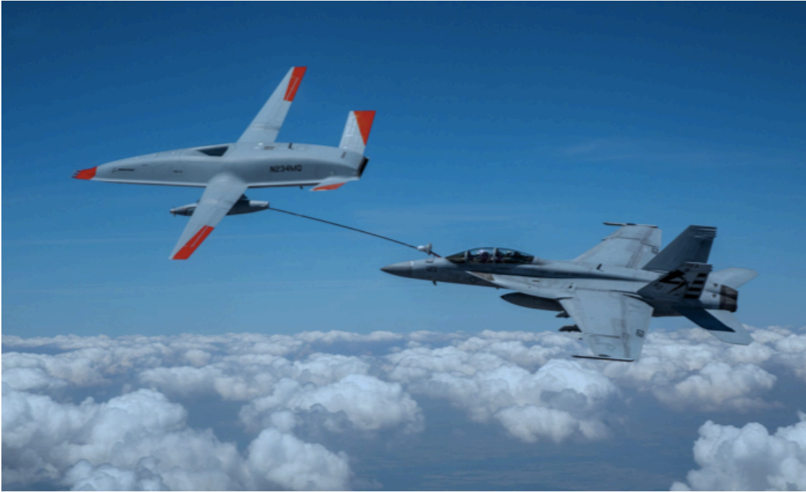
An unmanned Boeing MQ-25 T1 Stingray test aircraft, left, refuels a manned F/A-18 Super Hornet, June 4, 2021, near MidAmerica Airport in Mascoutah, Illinois. (U.S. Navy photo courtesy of Boeing)
