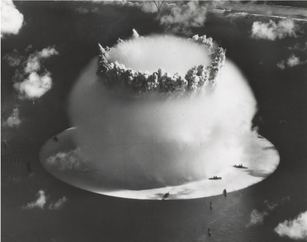
The Wilson cloud from test Baker, situated just offshore from Bikini Island at top of the picture. (Source: U.S. Army Photographic Signal Corps/Public Domain)
